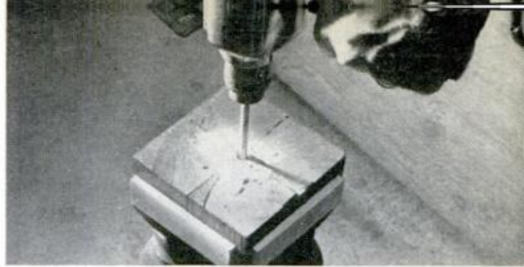
HOLES are drilled through the centers of the top and the base of the column. Use a 1/4-in. drill bit
